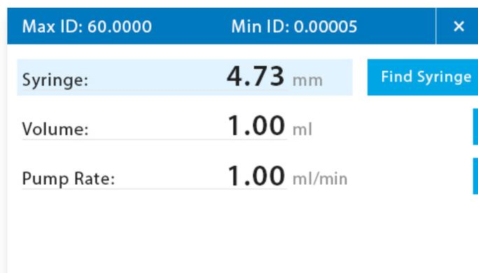
The screenshot shows the 'Basic Mode Screen' with a blue header bar containing 'Max ID: 60.0000' and 'Min ID: 0.00005' with a close button (X). Below the header, there are three input fields: 'Syringe:' with a value of '4.73 mm' and a 'Find Syringe' button; 'Volume:' with a value of '1.00 ml'; and 'Pump Rate:' with a value of '1.00 ml/min'.
