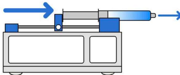
A syringe pump is a small, positive-displacement pump used to gradually transfer precise volumes of fluid. All Chemyx Fusion-series syringe pumps are driven via a stepper motor. This stepper motor precisely turns a lead screw that is threaded through a pusher block, which causes the pusher block to move. When the pump is in infusion mode, the pusher block pushes against the plunger of a secured syringe, causing the fluid to be ejected at an accurate and precise rate.
