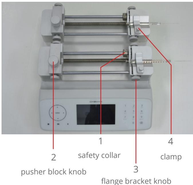
5. Loosen the bracket clamp knob for the plunger retaining bracket and adjust the gap such that the plunger cap of the syringe may fit.
