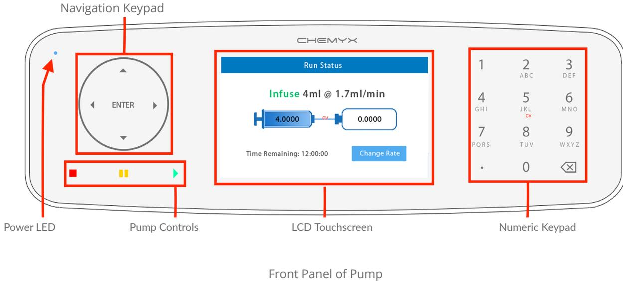
The Fusion Series uses a bright, 4.25", capacitive LCD touchscreen with an intuitive graphical user interface (GUI) for setting up detailed pump run methods. Buttons and entry fields within the GUI are all selectable using the touchscreen. As a capacitive LCD touchscreen, the interface can be operated with any object, not just the touch of a fingertip. Selecting elements by touch only requires a small amount of pressure; however, please do not use sharp objects as they may damage the screen.
