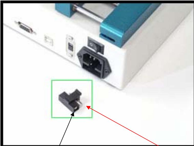
There are 2 fuses in the fuse holder. The exposed fuse in the back is the fuse that is being currently used. In the event of a power surge **this fuse will be the broken fuse.**
