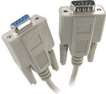
DB9 Serial Cable Male to Female – Straight through configuration. Do not purchase a "Null Modem," "crossover," or "crossed over" cables.
